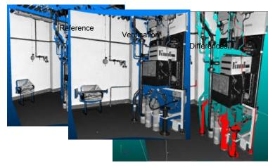
Laser Surface Mapping for Containment Versation (LMCV)
